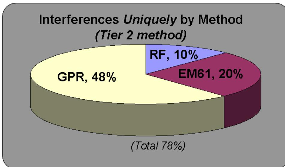
Figure 3. Pie chart showing the percentage of interferences *uniquely* designated by a given geophysical method for the same 23 Tier II surveys at the INL as shown in Figure 2. Note the sum of percentages here is only 78% as the interferences designated by more than one method were excluded. This result is worth noting in that it indicates that without the GPR
