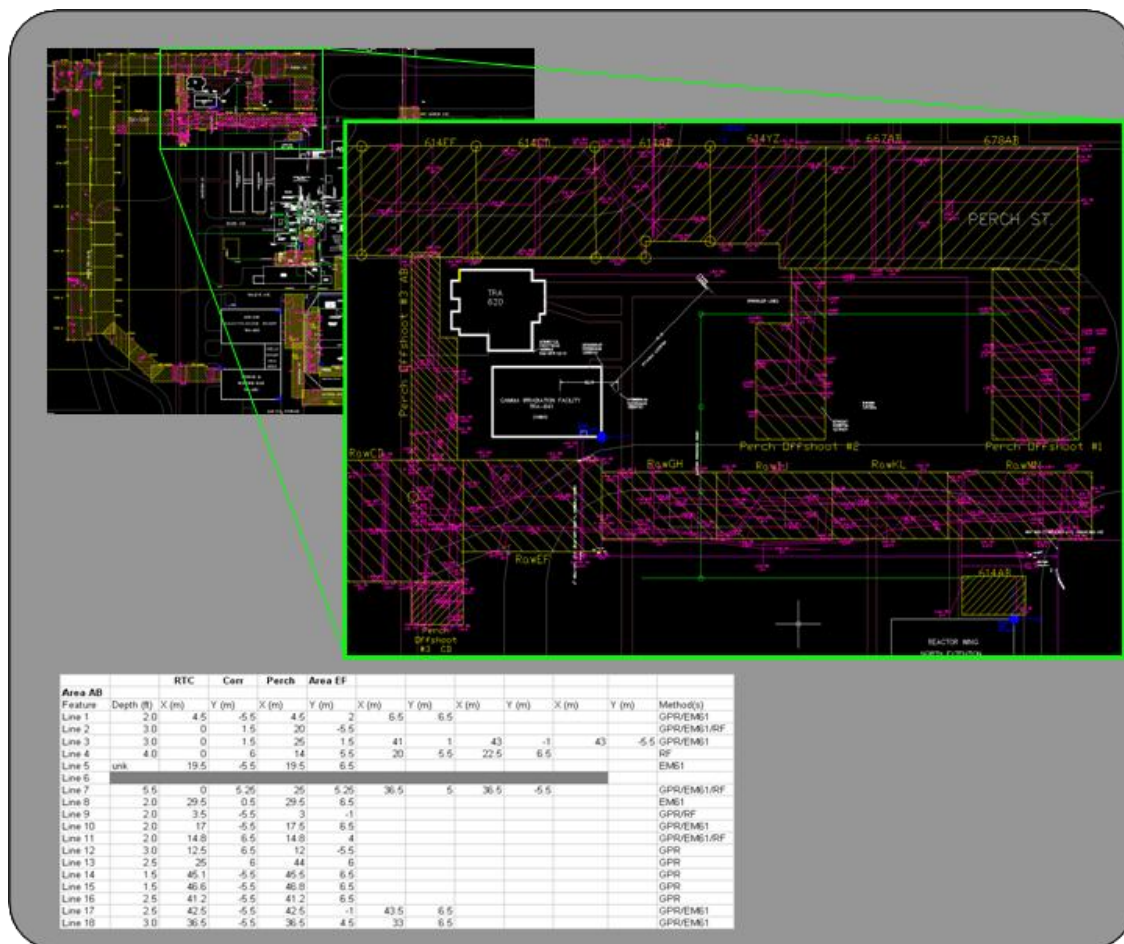
Figure 5. An example of a Subsurface Survey result in drawing form and a listing of the interferences designated in one survey area from the drawing. Note the drawing includes
