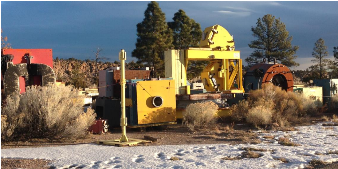
Photo 1 - TA-53 Magnet Pad – hundreds of tons of copper, steel and aluminum exposed to elements and subject to environmental review as a non-point source of water pollution.
