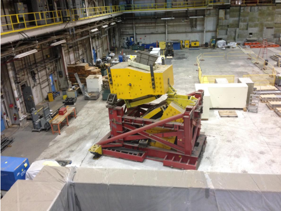
Photo 2 – EPICS Spectrometer in Area A – over 200 tons of magnet and cold-rolled steel encumbering projected new mission workspace.
