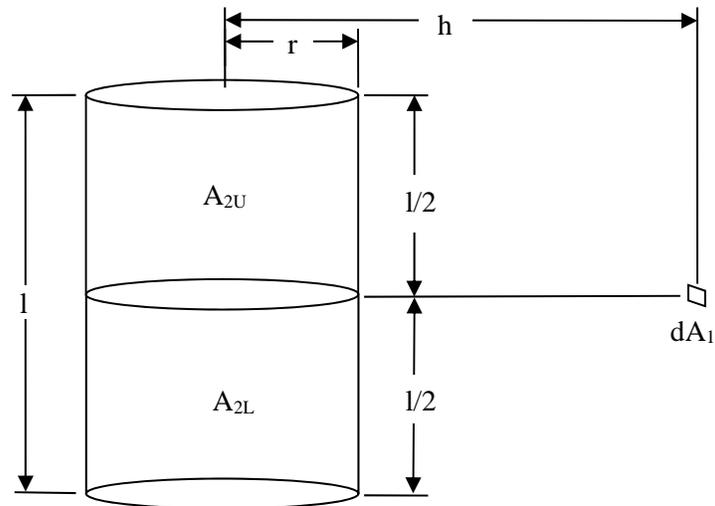
**Figure 2. Adaptation of View Factor Geometry for a Fire Model**
