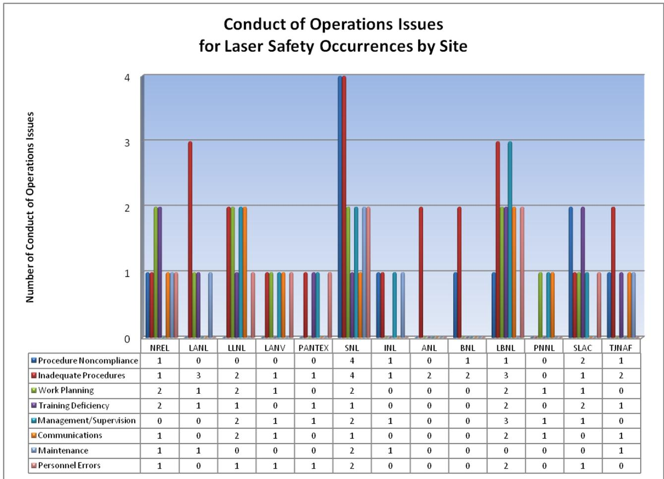
The analysis of conduct of operations execution issues indicates that Sandia National Laboratories had the most occurrences in which either procedures were inadequate or were not followed.
