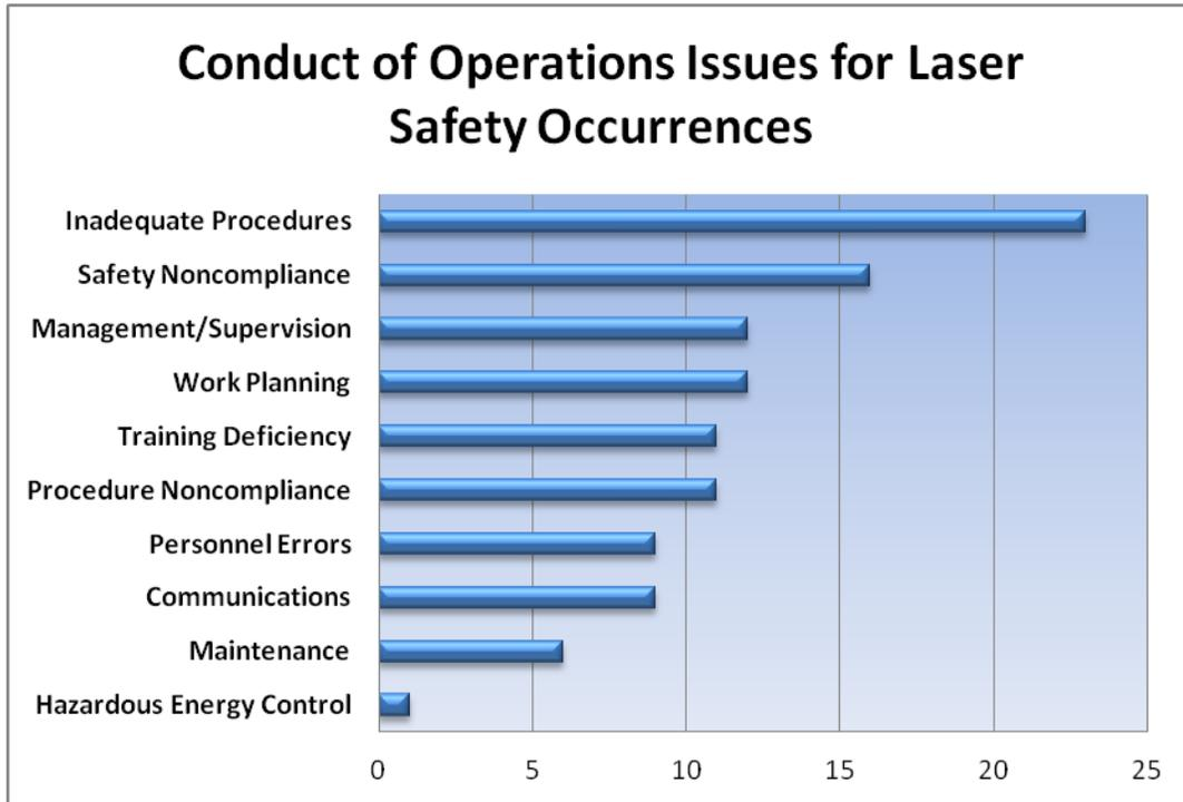
The data in Figure 8 shows that Inadequate Procedures was the most significant issue followed by Safety Non-Compliances. In some occurrences, evolutions were performed in which there was no procedure or the procedure did not address important safety issues.
