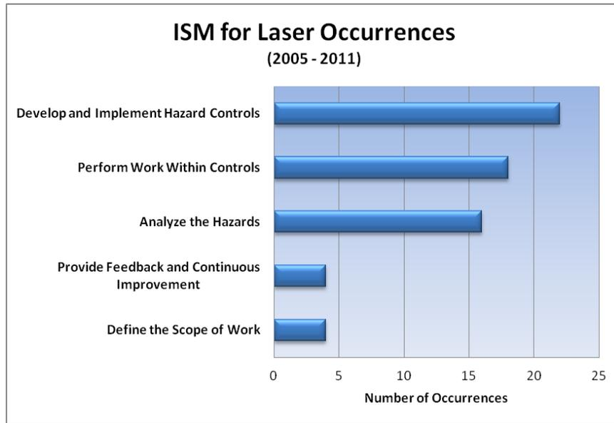
The ISM codes, which were assigned by the sites, show that Developing and Implementing Hazard Controls was the top code, followed by Performing Work Within Controls. Defining the Scope of Work was not seen as a major cause of laser occurrences.
