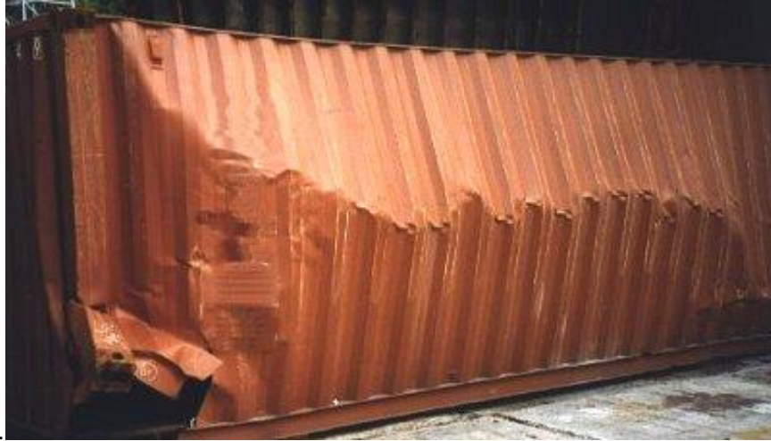
Figure 6-1. Damaged Freight Container from Internal Contents
