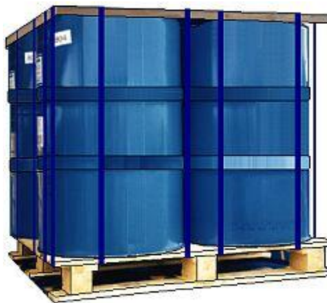
Figure 6-4. Properly palletized drums
