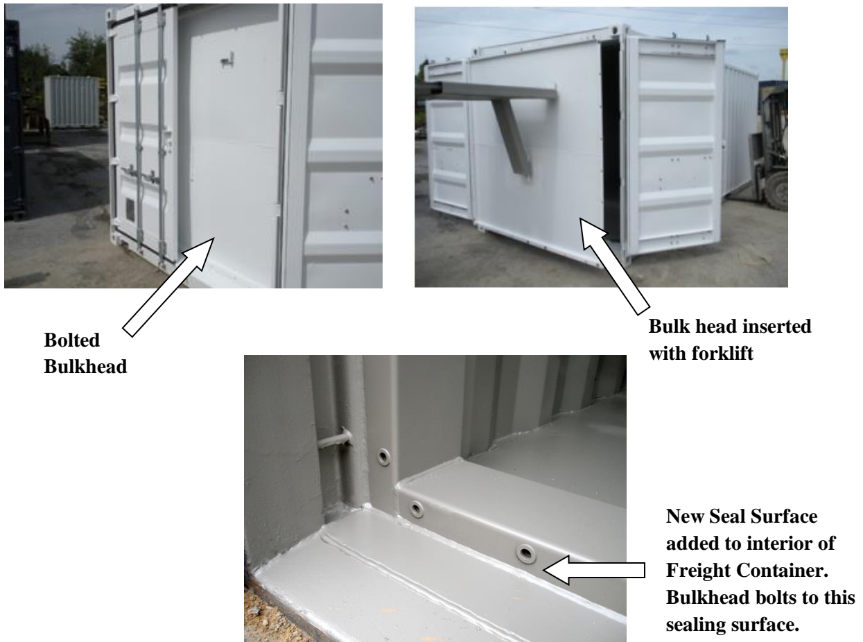
Figure L-4. Bulkhead with bolted closure
