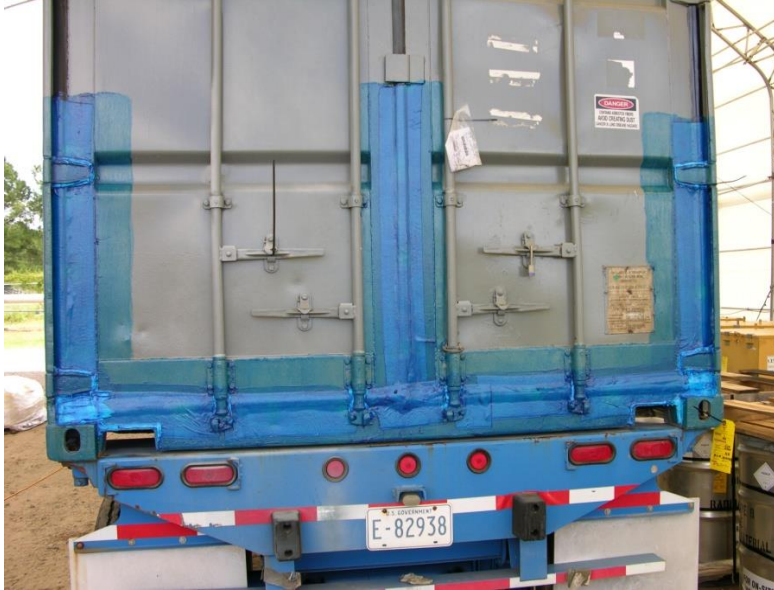
Figure L-1. Flexible membrane material sealed over outside of door joints.
