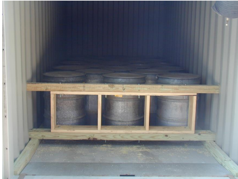
Figure 6-3. Drums that are properly blocked and braced
