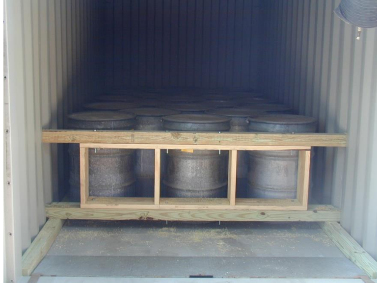
Figure 6-3. Drums that are properly blocked and braced
