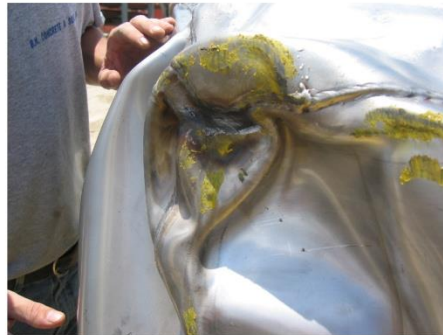
Figure 10. Deformation in waste box after CG/corner 1.2 m drop (major deformation).
