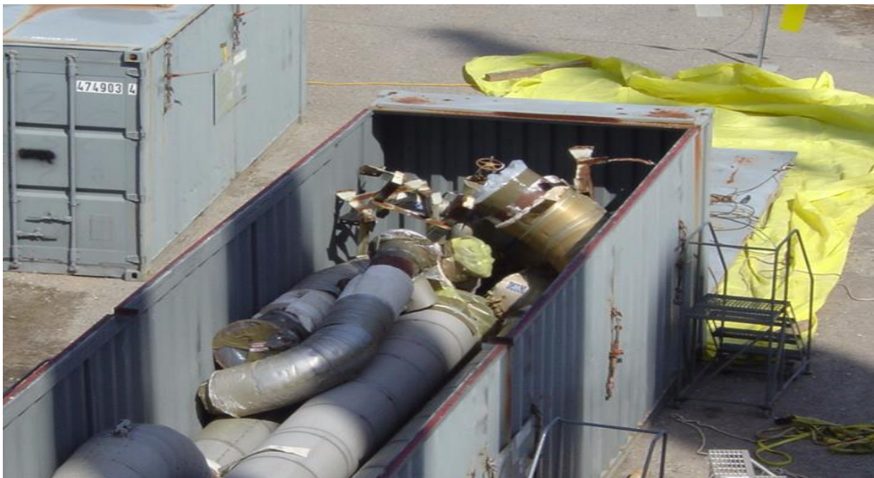
Figure 3-1. Piping with internal contamination and openings sealed with plastic and tape. This content can be considered non-dispersible.
