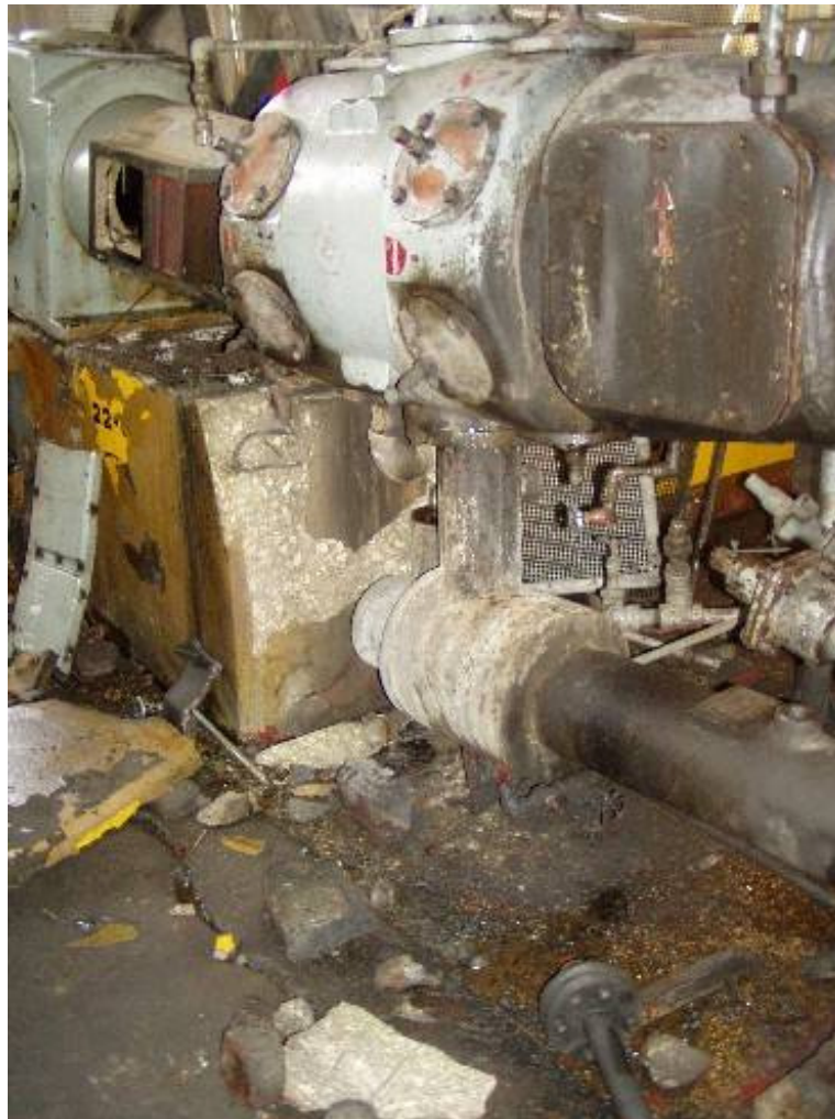
Figure 14.1 Ruptured horizontal compressor
