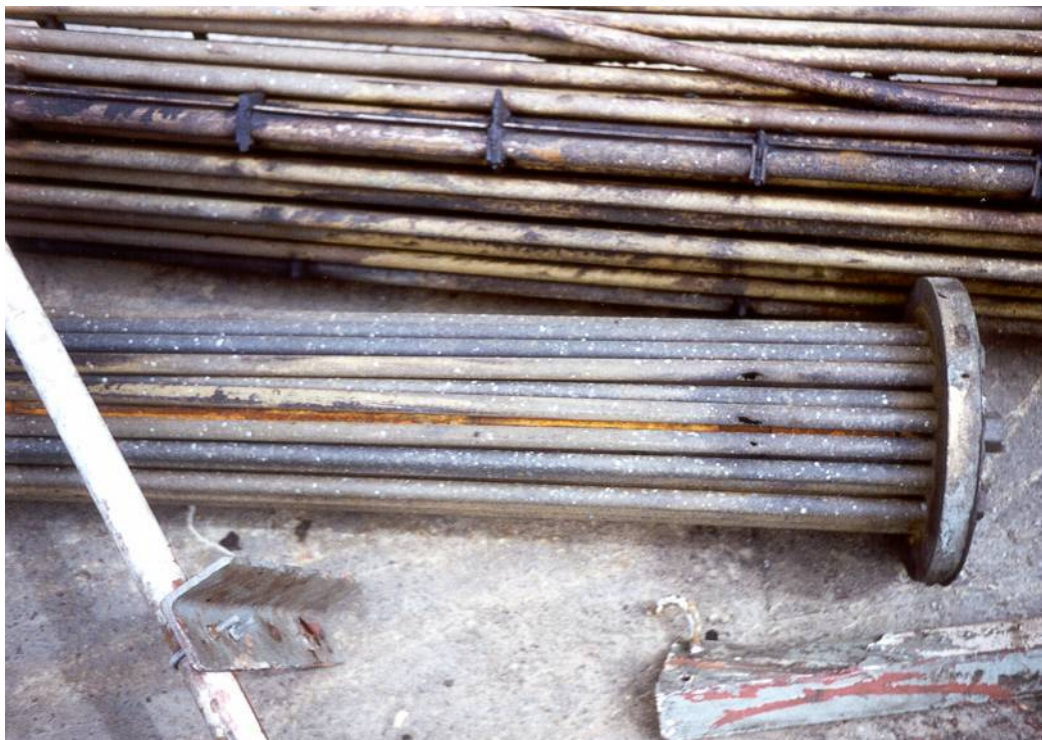
Figure 19.2 Holes in heat exchanger due to fretting corrosion, widened by pressurised flow.
