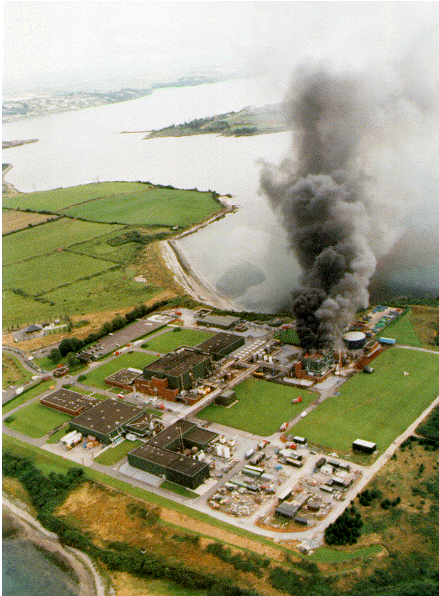
Figure 15.3 Explosion results from dry distillation of solvent and residue
