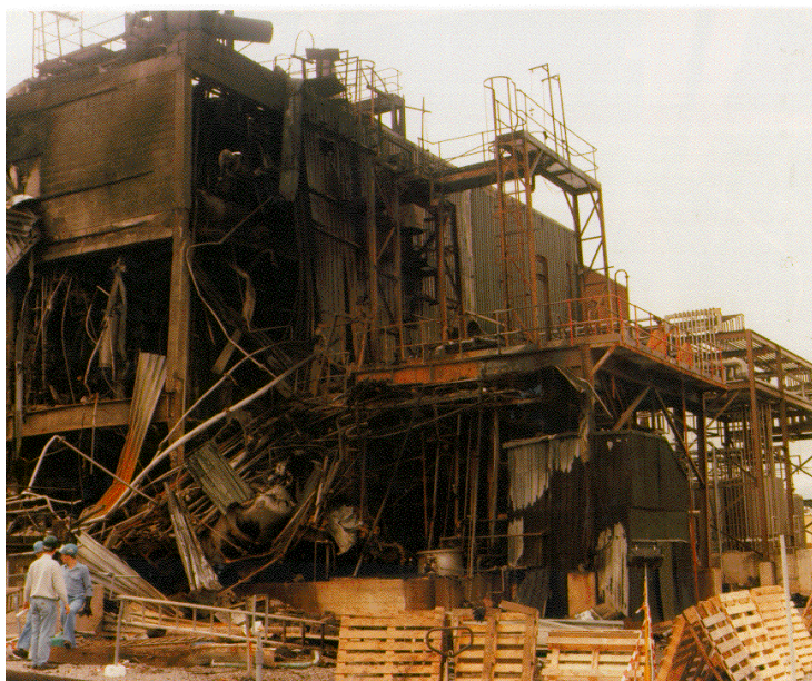
Figure 15.2 Explosion results from dry distillation of solvent and residue
