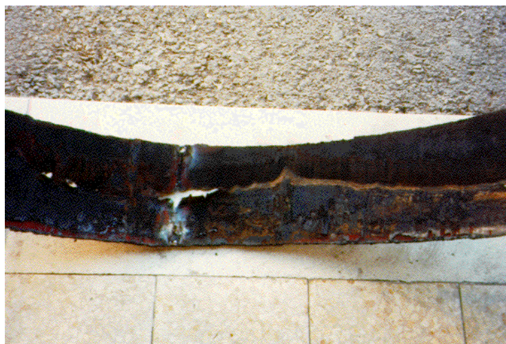
Figure 7.7 Section from a pipe wall damaged by cavitation on an expansion section
