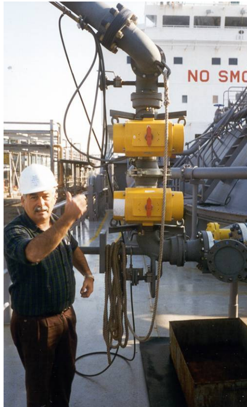
Figure 11.3 High integrity loading arm coupling, designed by the author.
