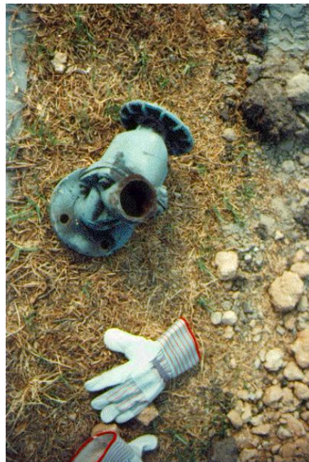
Figure 7.6 A cast iron valve, broken by impact
