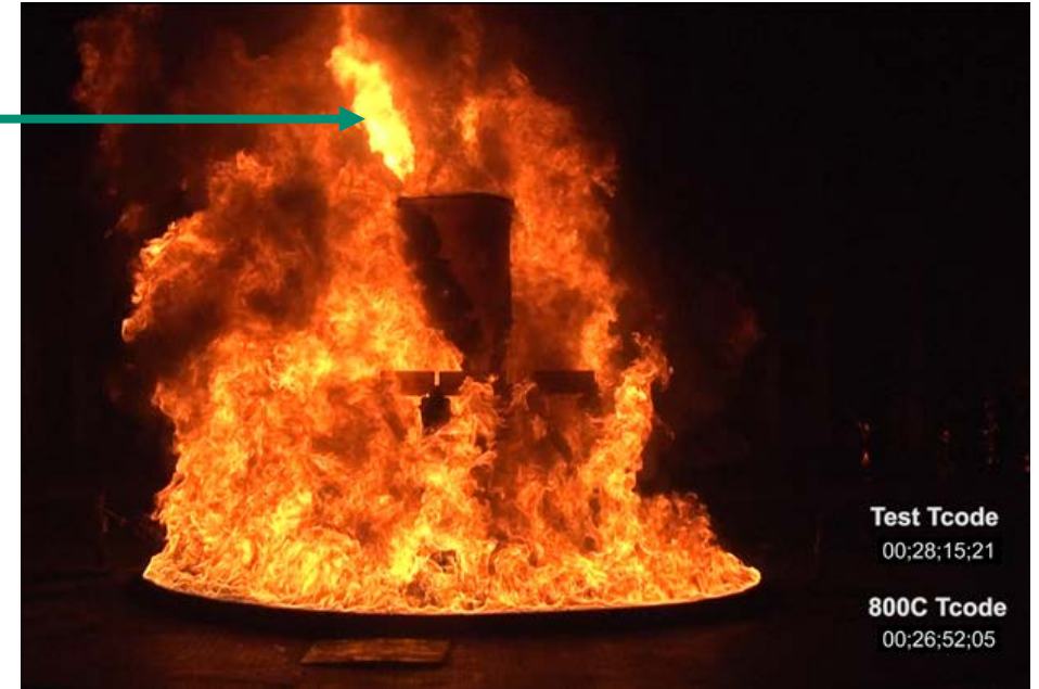
7A drum after 30-minute fully engulfing pool fire
