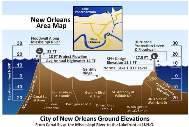
City of New Orleans Ground Elevations From Canal St. at the Mississippi River to the Lakefront at U.N.O. Vertical cross-section of New Orleans, showing maximum levee height of 23 feet (7 m) at the Mississippi River on the left and 17.5 feet (5 m) at Lake Pontchartrain on the right.
