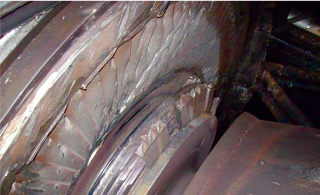
Figure 1. Last stage blading roots and diaphragm (a stationary component that directs steam into the last-stage blading).
