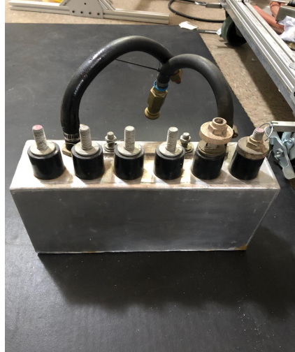
Figure 13. Six capacitors in a single enclosure.
