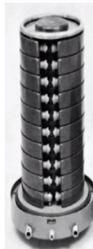
Figure 16. example of a small Marx stack of 10 modules
