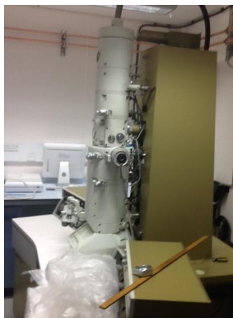
Figure 14. Transmission electron microscope, 300 V high-voltage coaxial cable.
