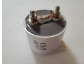
Figure 10c. Capacitor with a drain wire in place between the two terminals.
