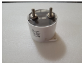
Figure 10a. Example 2. An isolated, unsafe capacitor.
