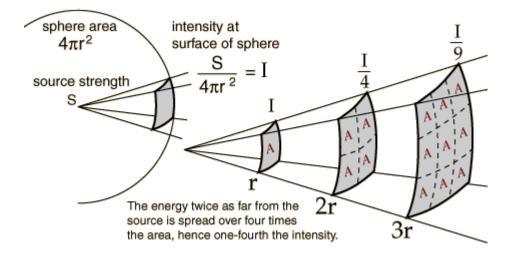
The lines represent the flux emanating from the source. The total number of flux lines depends on the strength of the source and is constant with increasing distance. The density of flux lines is inversely proportional to the square of the distance from the source because the surface area of a sphere increases with the square of the radius. Thus the strength of the field is inversely proportional to the square of the distance from the source. The energy twice the distance from a given source is
