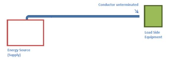
**Condition 2:** LOTO does apply when conductors are unterminated from the equipment (load side).
