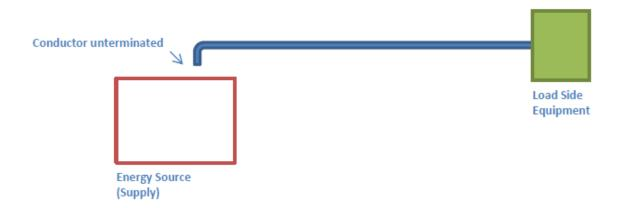
**Condition 1:** LOTO does not apply when the conductors are unterminated from the source(s) of energy (supply side). To meet the intent for Condition 1, entire removal of the conductor or removal of a section of the conductor such that the conductor cannot be re-terminated is required.
