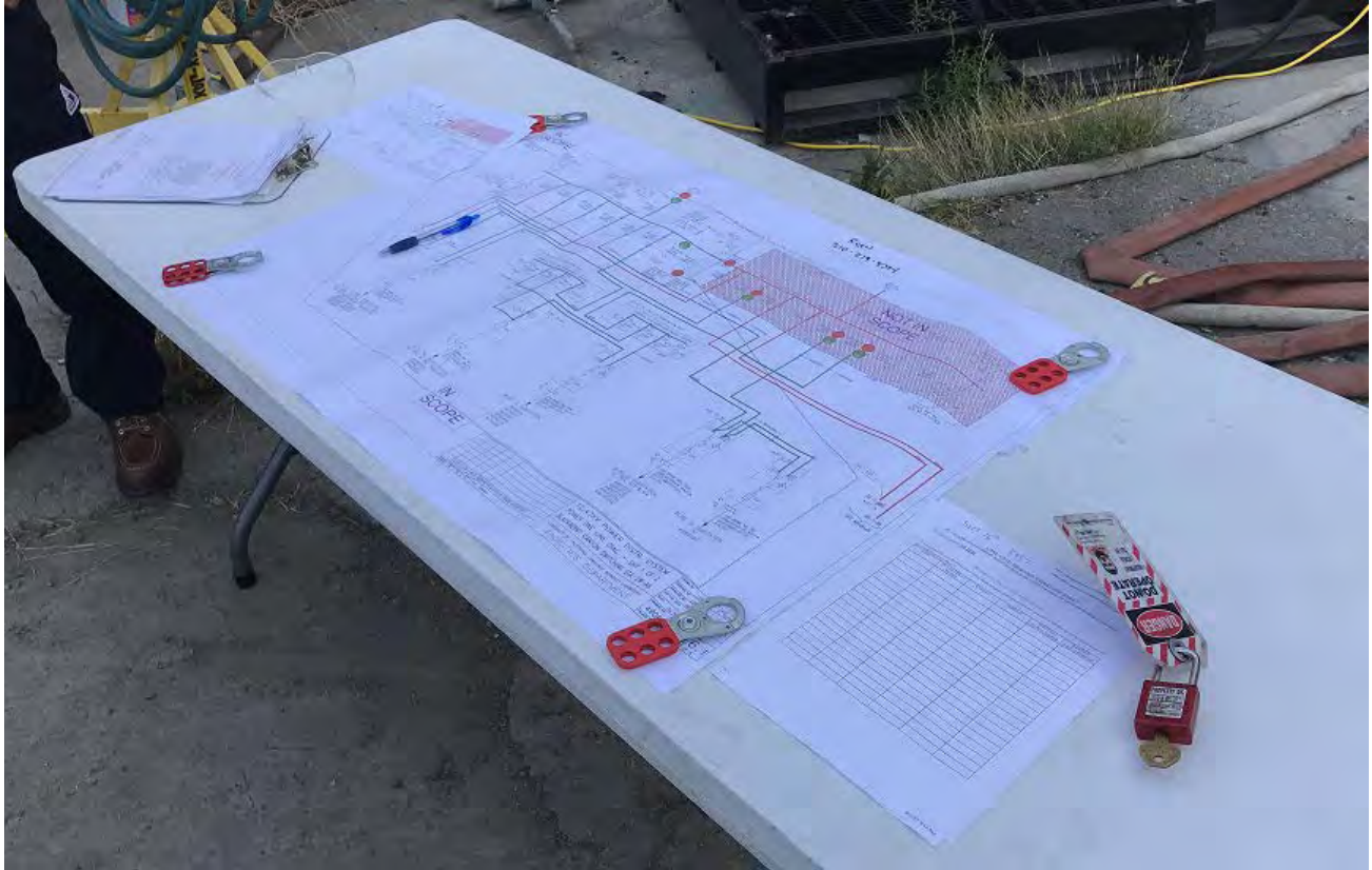
Figure 7A – One line drawing delineating LOTO isolations, grounding device locations and work scope located at work site
