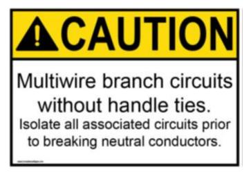
8. A branch circuit cable or conduit enters a panel with more ungrounded conductors than neutral conductors, and the ungrounded conductors terminate at single pole circuit breakers.
