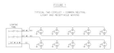
COMMON NEUTRAL CARRIES THE DIFFERENCE IN CURRENT (UNBALANCE) BETWEEN CIRCUIT 1 AND 3.
