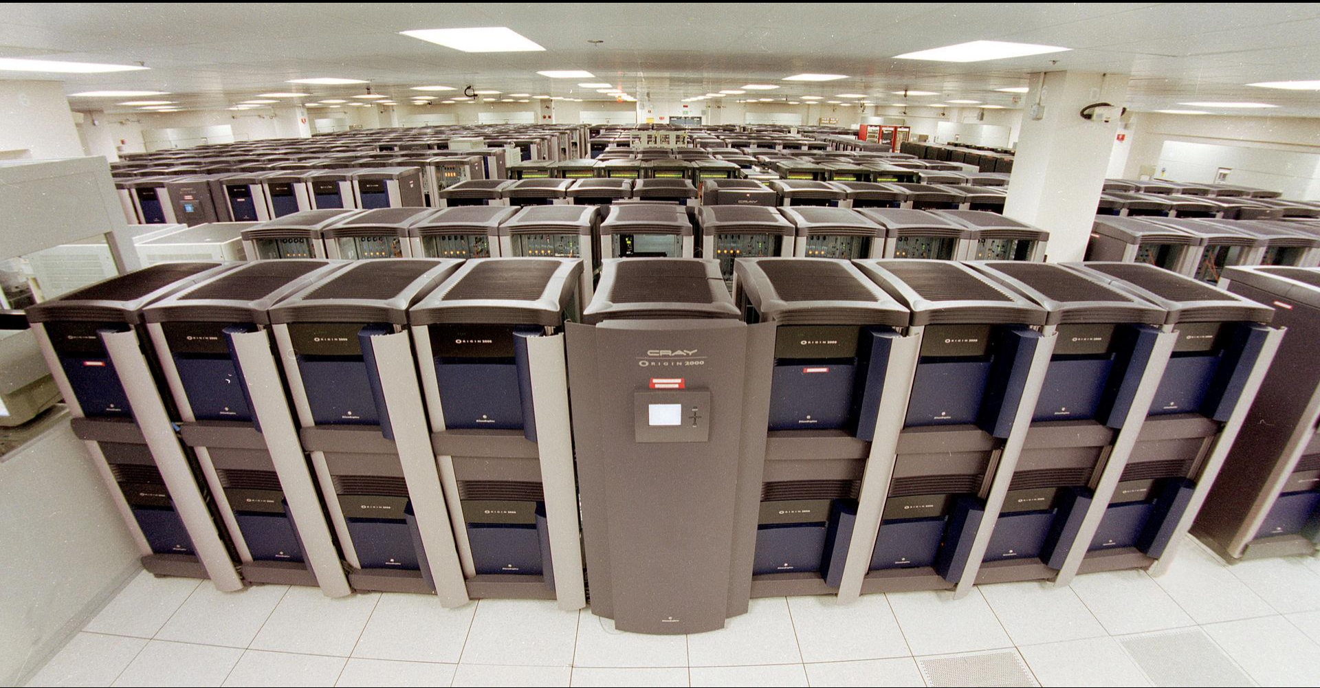
ASCI Blue Mountain (1998-2004), LANL's first large-scale cluster computer. 3 teraflops performance equaled 19-thousand Cray-1 systems.
