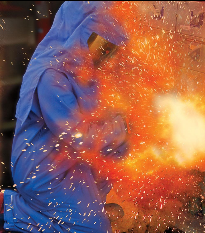
Arc flash event with proper arc rated PPE.
