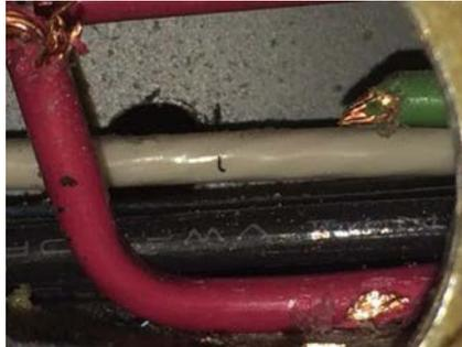
Just recently a carpenter cut through a non-metallic cable with a reciprocating saw while cutting out a damaged piece of roof framing. Even though it was evident there were electrical cables in the area and he had felt around for any existing wiring prior to cutting, it was not enough to keep the cable from getting cut and tripping a circuit.
