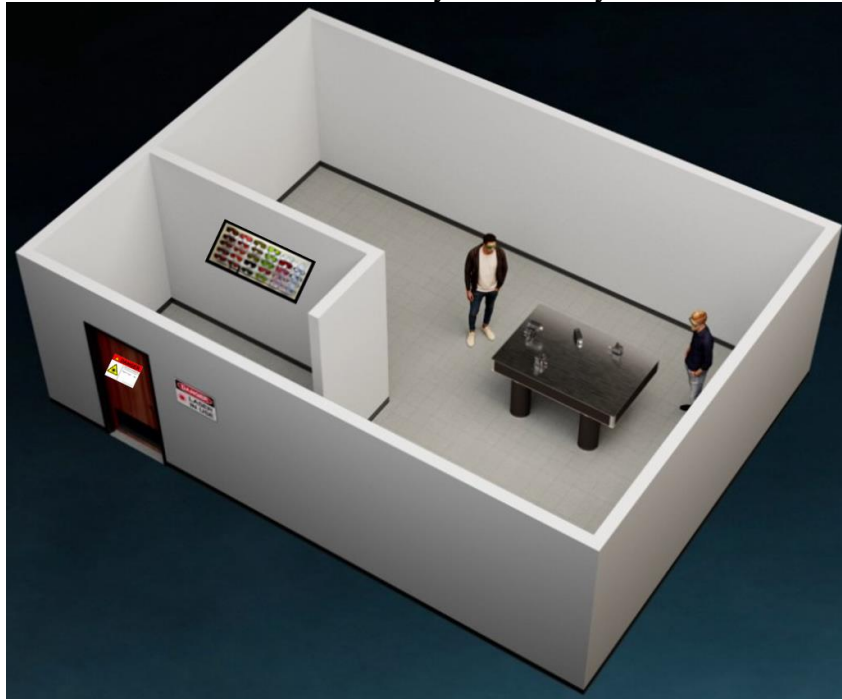
Figure 1-1. The Laser Controlled Area (LCA) is bounded by four walls. On the front wall is the entry door with an associated laser hazard sign and an electronic laser status warning device.
