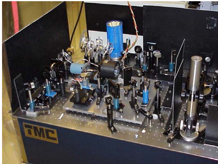
Figure 2. Perimeter guards with beam blocks
