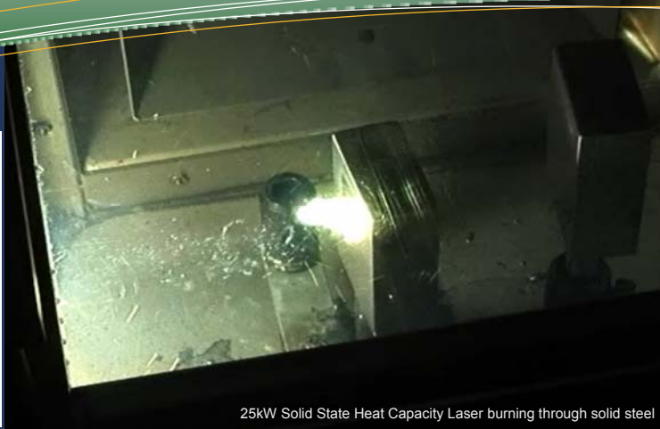
25kW Solid State Heat Capacity Laser burning through solid steel
