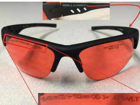
Figure 4. Wrong Eyewear for this task – "visible alignment" imprinted on left arm.
