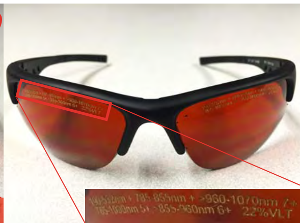
Figure 5. Proper Eyewear for this task.
