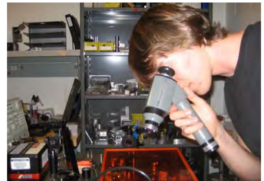
Figure 1. Incorrect use of IR viewer (no LPE)
