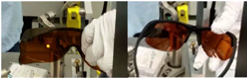
Figure 7. Fluorescing spot on left pair while right pair shows no effect
