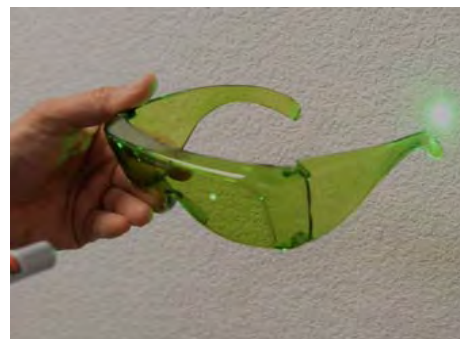
Figure 1. Wrong eyewear transparent to laser beam
