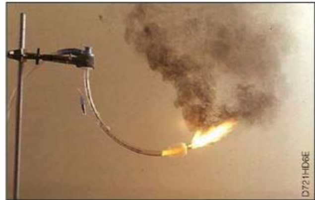
Figure 2. Demonstration of rocket-like flames shooting from a tracheal tube caused by laser ignition of the tube with 100% oxygen flowing. Image provided courtesy of ECRI Institute.
