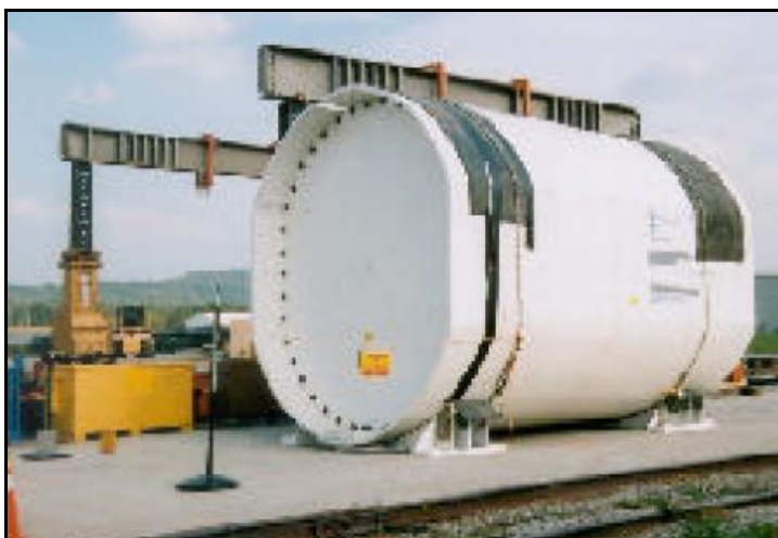
Figure 2-6. The Concentrator Feed Makeup Tank Shipping Container (WVDP photo)
